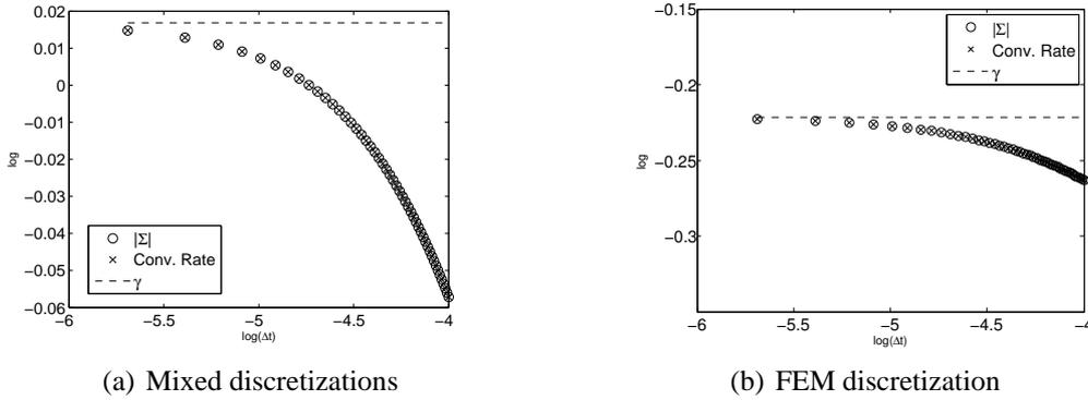
Figure 5: Case 4 from table 1. Comparison between  $\gamma$  (left) and  $\gamma_{\text{FEM}}$  (right). The curves are restricted to the discrete values  $\Delta t = 1e - 4/50, 2 \cdot 1e - 4/50, \dots, 50 \cdot 1e - 4/50$  and  $\Delta x = 1/20$ . Observe that  $\gamma > \gamma_{\text{FEM}}$  and in particular,  $\gamma \approx 1.74\gamma_{\text{FEM}}$ .
