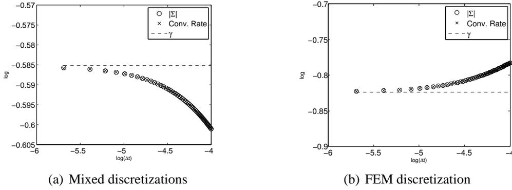
Figure 4: Case 3 from table 1. Comparison between  $\gamma$  (left) and  $\gamma_{\text{FEM}}$  (right). The curves are restricted to the discrete values  $\Delta t = 1e - 4/50, 2 \cdot 1e - 4/50, \dots, 50 \cdot 1e - 4/50$  and  $\Delta x = 1/20$ . Observe that  $\gamma > \gamma_{\text{FEM}}$  and in particular,  $\gamma \approx 1.74\gamma_{\text{FEM}}$ .
