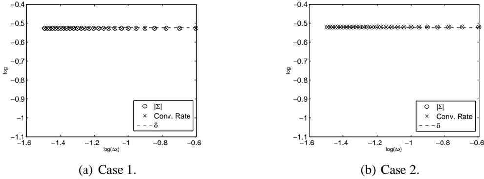
Figure 3: Cases 1 and 2 from table 1. The curves are restricted to the discrete values  $\Delta x = 1/3, 1/4, \dots, 1/30$  and  $\Delta t = 100$ . One observes how  $\delta$  describes the behaviour of the convergence rates when we enforce the condition  $\Delta t/\Delta x^2 \gg 1$ .
